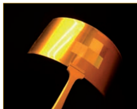
Flexible OrmoStamp® on nickel backplate (Courtesy of PSI, Switzerland)
